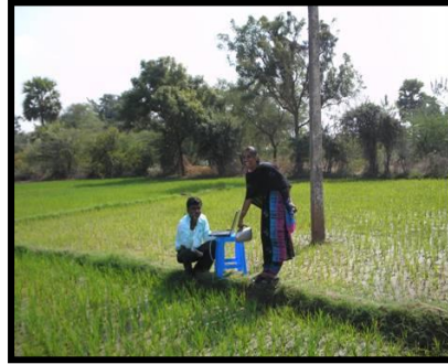
Photo 2: Using a handheld spectro-radiometer ( Analytical Instruments Ltd. USA ) to collect spectral signature from paddy field at early growth stage in Gollapalli village.
