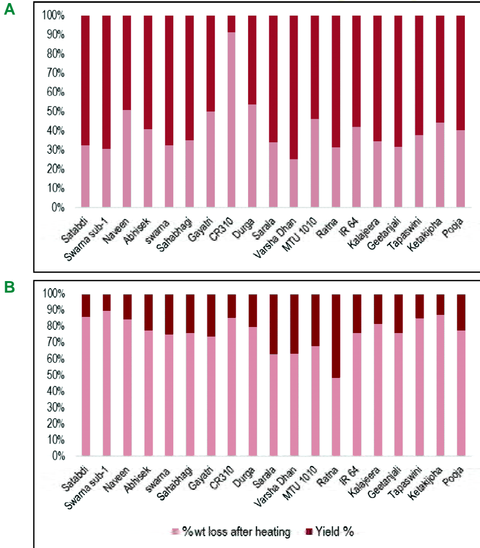
Fig. 3. Yield and weight loss of the Biochar produced from nineteen rice cultivars (A. 300 C for 2 hours, B. 300 C for 4 hours)
