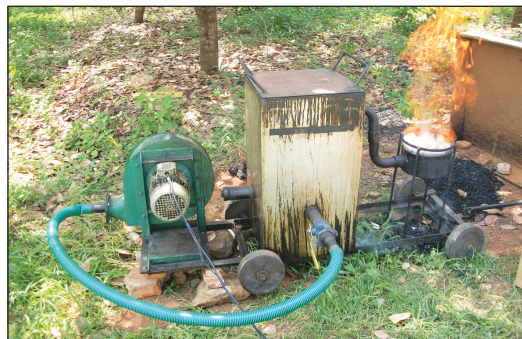
Gasification process of cashew shell cake based updraft gasifier
