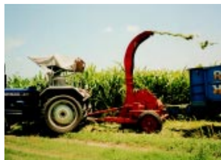
Tractor-mounted fodder harvester in a single operation can harvest, chop and load the chopped fodders like maize, pearl millet, oat etc. in the trailer attached to the machine
