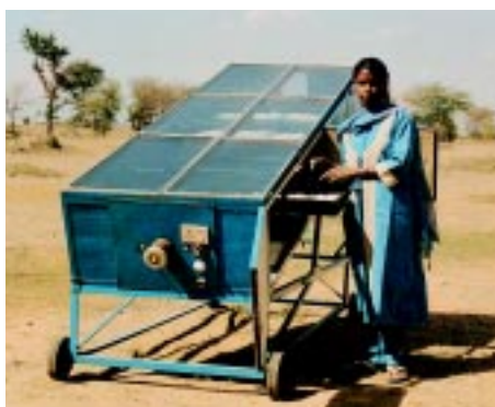
Step type solar cocoon stifter was found to be at par to stifled cocoons in the conventional ovens
