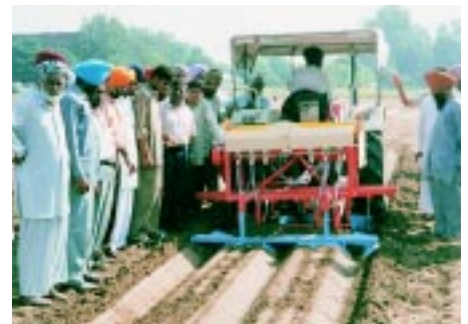
Tractor-mounted raised bed planter saves 20% in seed rate, about 30% in fertilizer and 34% in irrigation water requirement besides getting higher yields
