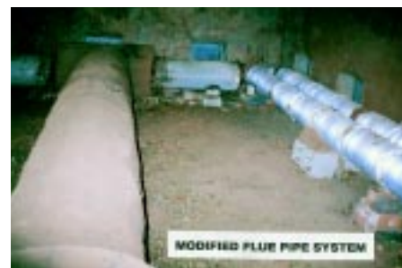
Modified flue-pipe system of tobacco-curing, designed by the TIDE, Bangalore, gives about 25% saving in wood fuel consumption in Karnataka compared to conventional flue-pipe system
