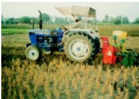
Tractor-mounted till planter performs better in silt clay loam soil where one pass of tractor-mounted disc harrow is added in the treatment
