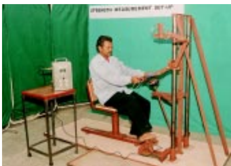
Strength measurement set-up with both hands (top), in paddle operation in sitting posture (bottom)
