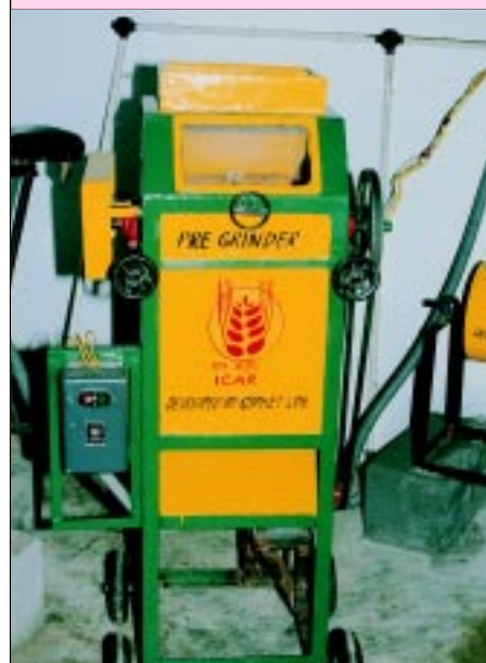
A pre-grinder for oilseeds of 100 kg/hr capacity has been developed at CIPHET, Ludhiana
