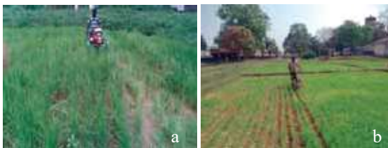
Fig. 5. Weeding in rice with two row wet land weeder (a) and single row dry land weeder (b).
