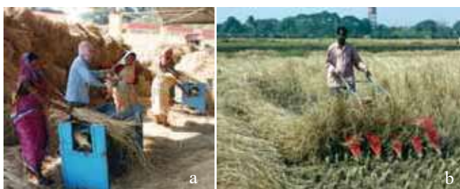
Fig. 7. Threshing by power operated drummy thresher (a) and harvesting by reaper (b).
