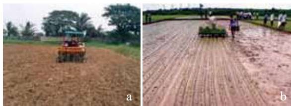
Fig. 4. Tractor drawn seed cum fertilizer drill (a) and self propelled eight row transplanter (b) in operation.
