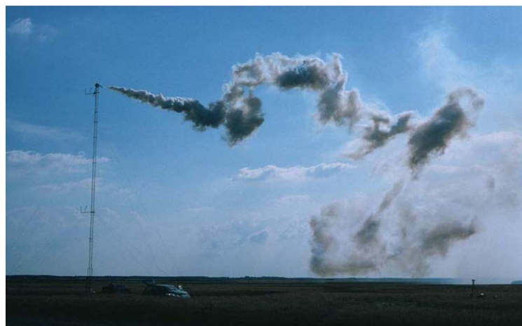
Dispersion experiments from an individual source for different atmospheric conditions, compare Figure 10.4. (T. Mikkelsen, personal communication)
