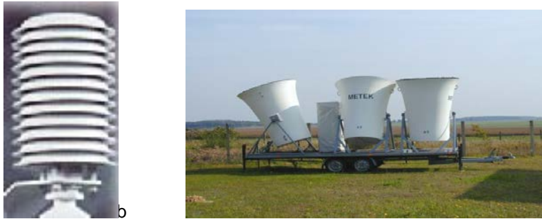
Figure 13.8 Screen ad protect for different instruments, temperature radiation screen, and SORAR enclosures.
