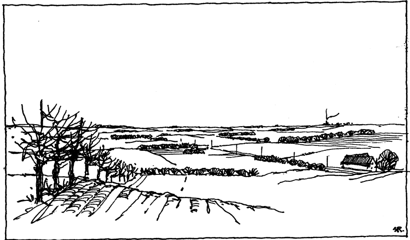
Figure 7.11. Terrain with roughness corresponding to roughness class 2, farm lands with wind breaks, the mean separation of which exceeds 1000 m, and some scattered build up areas, z_0 \cong 0.10 m. The terrain is characterised by large open areas between many wind breaks, giving the landscape an open appearance. The terrain may be flat or gently undulating. There are many trees and buildings. (Troen and Petersen, 1980)
