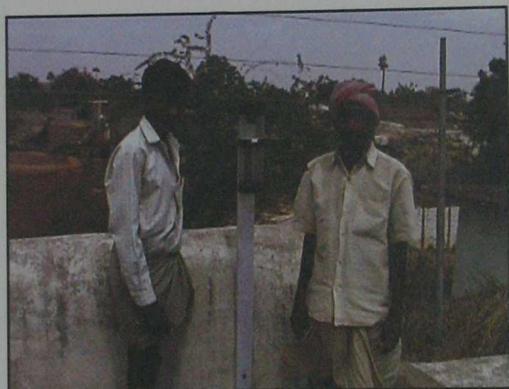
Fig. 5.14 Rain gauge (non-recording) on roof top of farmer's house
