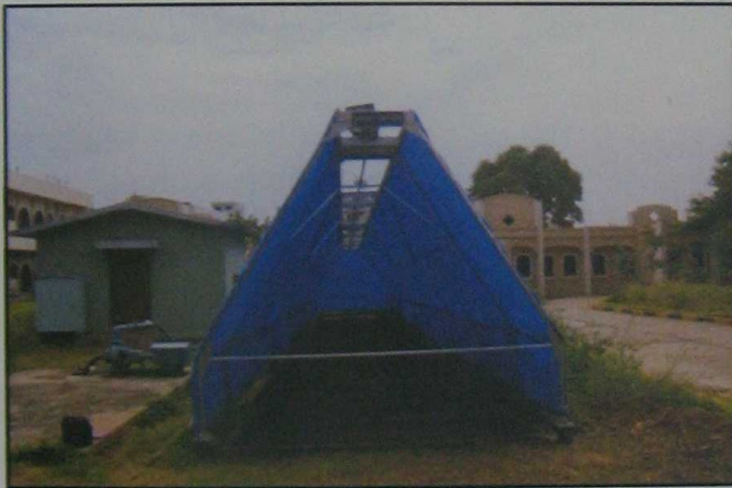
Fig. 6.1 Programmable rainfall simulator
