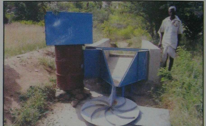
Fig.8.2 Stage level recorder installed in treated arable land
