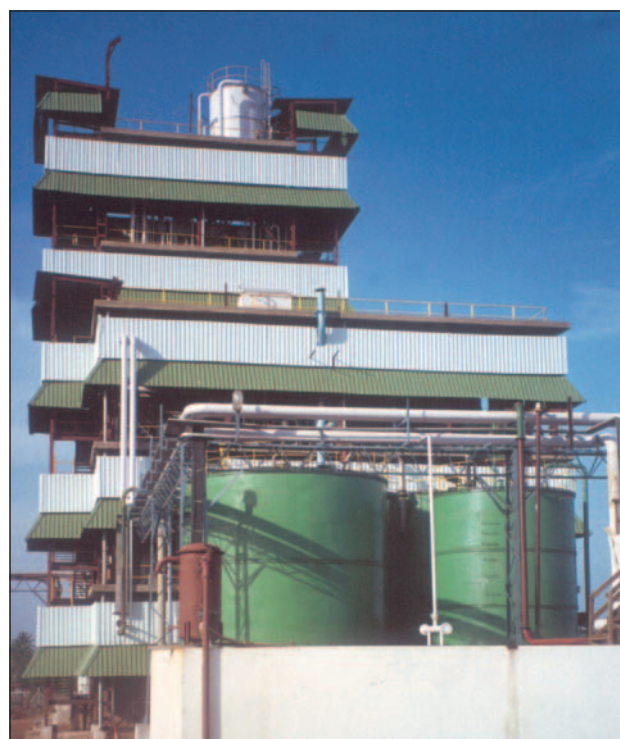
A 60 KL capacity fermentor used in pilot study on alcohol at M/s Renuka Sugars, Belgaum
