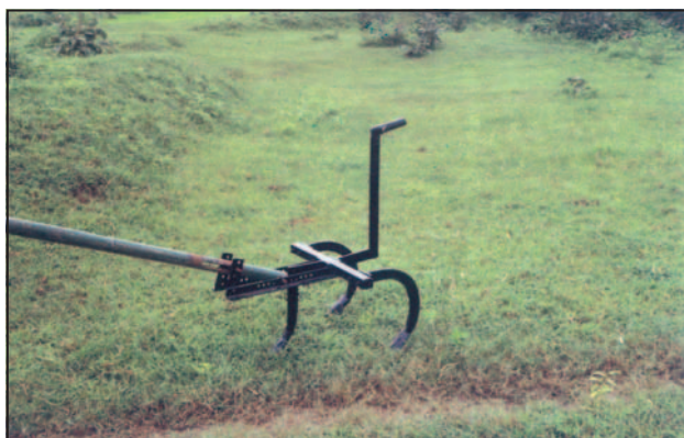
Trifal , a bullock drawn biasi implement developed by IGKV, Raipur
