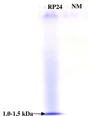
Fig. 5 SDS-PAGE of partially purified extract of RP24 (lane 1) and its negative mutant NM (lane 2)
