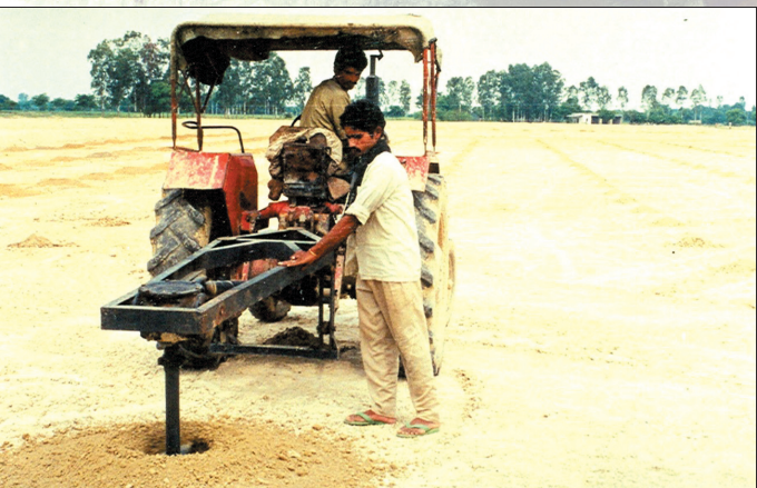
Auger-hole method for the afforestation of sodic soils
