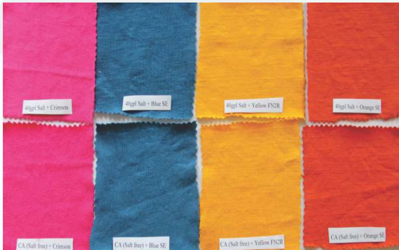
Fig. 2.18 Cotton fabrics dyed with and without salt using crimson HEXL reactive dye
