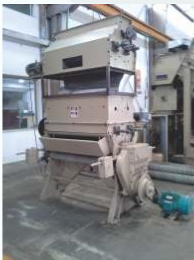
Fig. 2.1 Single Locking Cotton Feeder for Double Roller (DR) Gin
