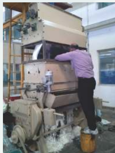
Fig. 2.1 Single Locking Cotton Feeder for Double Roller (DR) Gin
