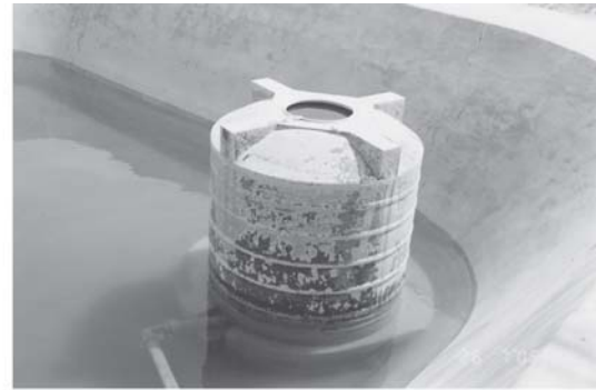
Neutralization of RSC water through gypsum tank for sprinkler irrigation
