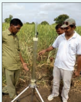
In-situ saturated hydraulic conductivity measured by using Guleph permeameter
