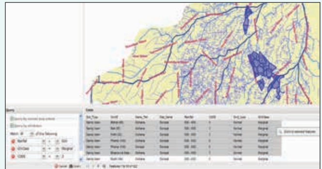
Fig. 24 : Online querying based on multiple layer attributes for identifying constraints in WYC Command
