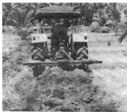
Fig.1. Power tiller and tractor operated turmeric digger
