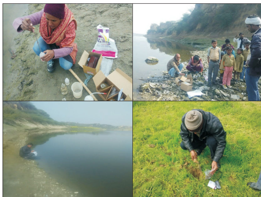
Photo 3.13: On site fixation of dissolved oxygen (Top) and identification of geographical coordinates of location with GPS (Bottom)
