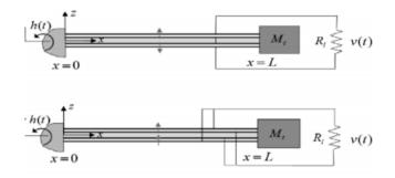
The governing equations of a bimorph piezoelectric energy harvester in the physical coordinates are given by
