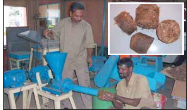
Fig. 2. Briquetting of shredded EFB
