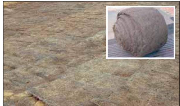
Fig. 4. Cooling pad from EFB fibres for environmental control over terraces
