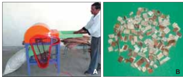
(A) Arecanut sheath shredder; (B) arecanut fodder
