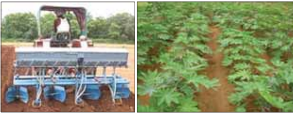
Ridge planter in operation and castor crop planted with ridge planter
