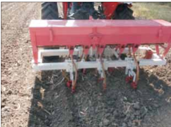
Tractor-operated multi row seed-cum-ferti drill
