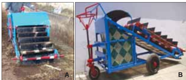
(A) Petrol-engine-operated dung collector; and (B) Electric-motor-operated dung collector
