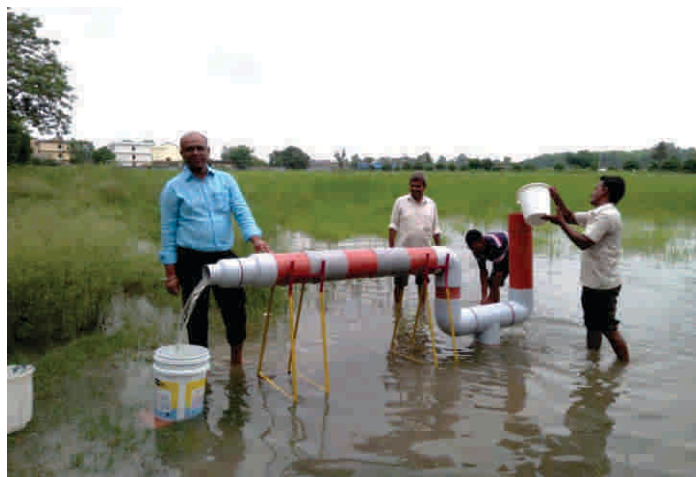
Plate 3.3.1. Filter assembly testing under field condition using runoff water
