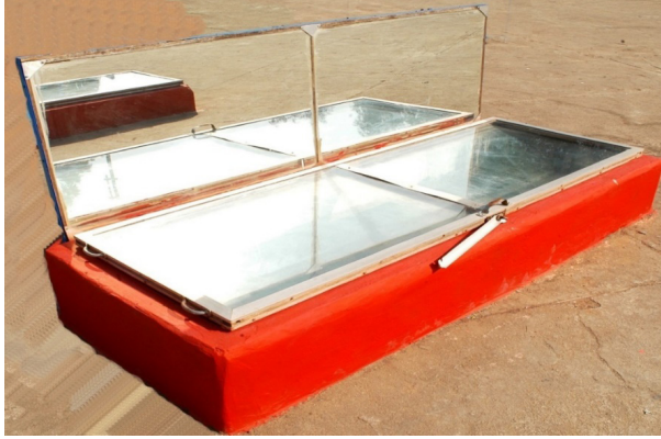
Fig. 2: Animal feed solar cooker installed in the field
