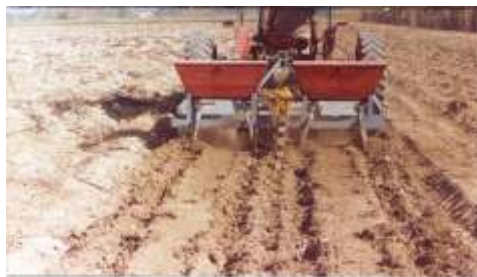
Fig. 11. Tractor-drawn stubble shaver for shaving stubble of sugarcane
