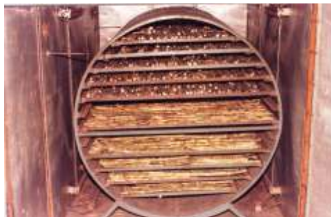
Fig.12. Moist hot air treatment unit (front view with doors open)
