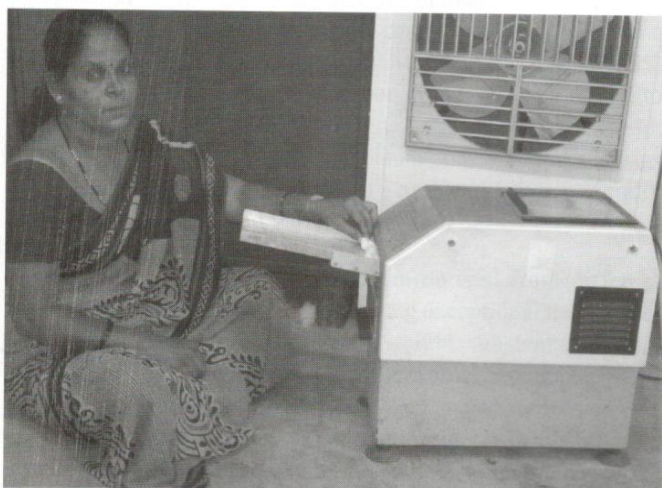
Figure 3: Opening of cotton lint samples using SDL Fibre Opener Blender
