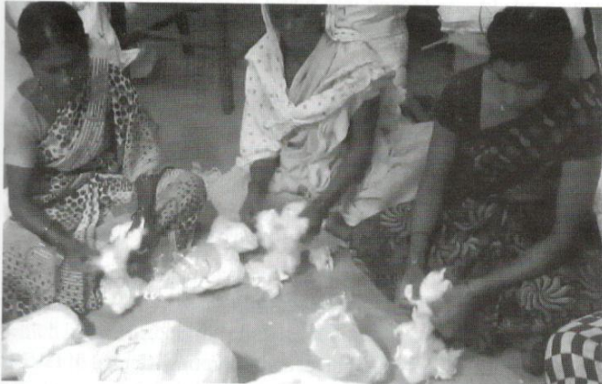
Figure 1: Opening of cotton lint samples manually by hand
