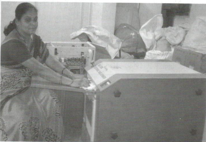
Figure 2: Opening of cotton lint samples using MAG Sitra Trash Analyzer
