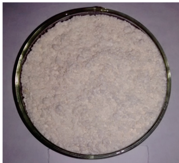
Fig. 4: FSO microcapsules prepared using TS-WPI coating combination under optimized process conditions
