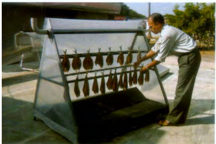
Fish drying in PVC tent dryer
