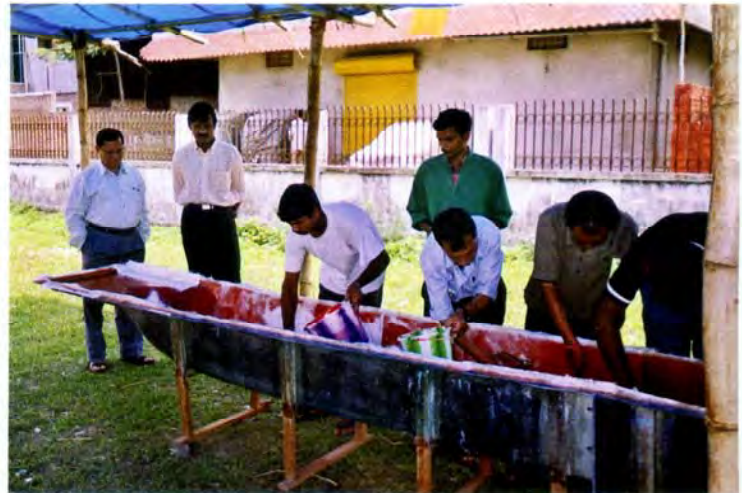
Fabrication of FRP canoes in progress
