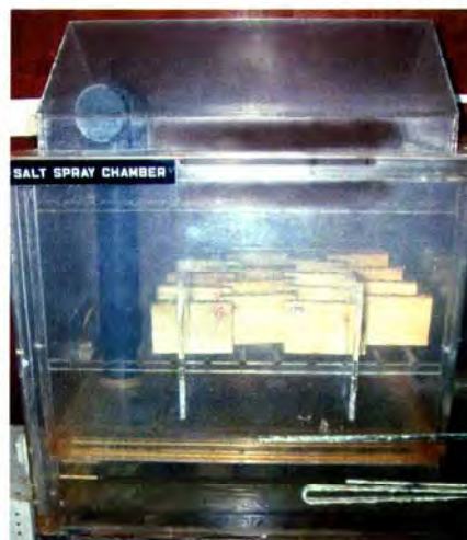
Panels in salt spray chamber
