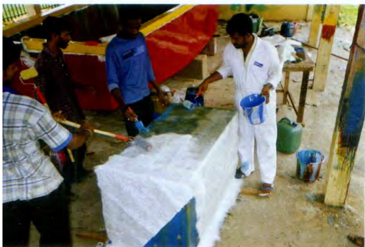
Fabrication of FRP fishing vessel
