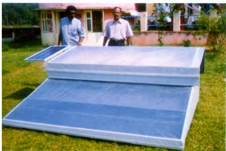
Forced circulation dryer under demonstration at Midnapur
