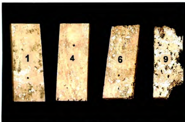
Borer attack within nine months
