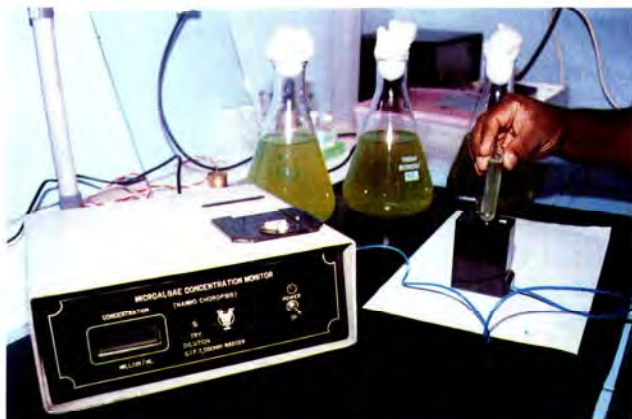
The micro algae concentration monitor – for measuring concentration of marine algae
