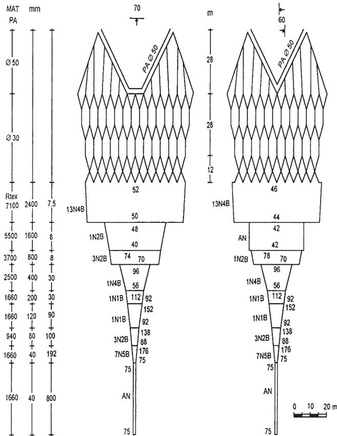
Figure 3. Design of 70.0 m midwater trawl
