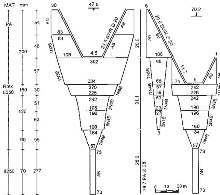
Figure 2. Design of 47.5 m bottom trawl.
