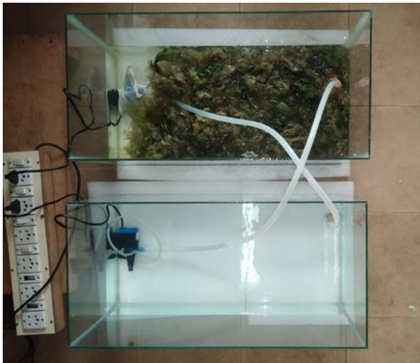
Fig 2: Seaweed based bioremediation unit
