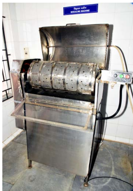
Fig.6 Fish descaling machine with variable drum speed
