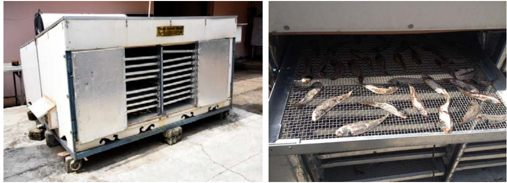
Fig.5. CIFT Solar-Cabinet Dryer with Electrical back-up
