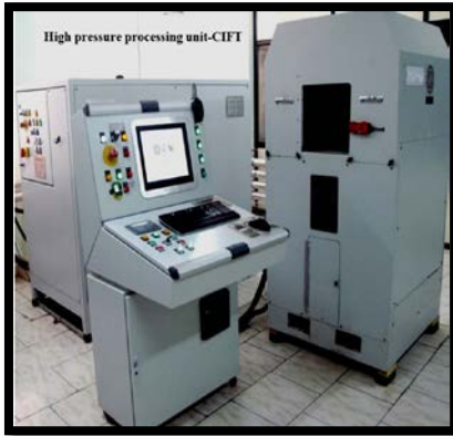
Fig.5. High pressure processing unit
