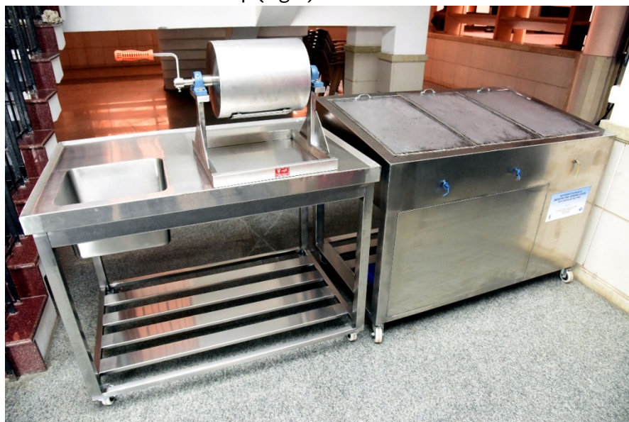
Fig.8 Refrigeration enabled Mobile Fish vending kiosk
