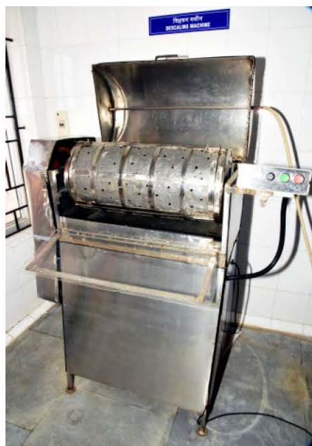
Fig.6 Fish descaling machine with variable drum speed
