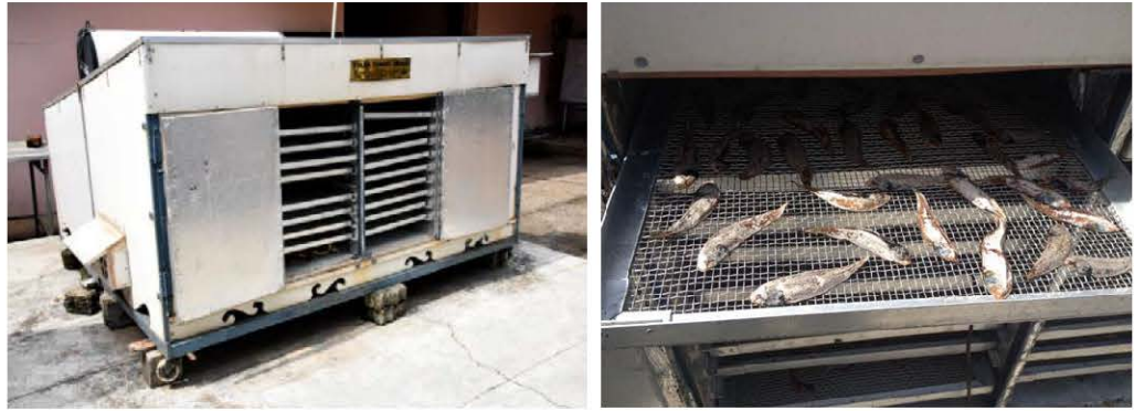
Fig.5. CIFT Solar-Cabinet Dryer with Electrical back-up
