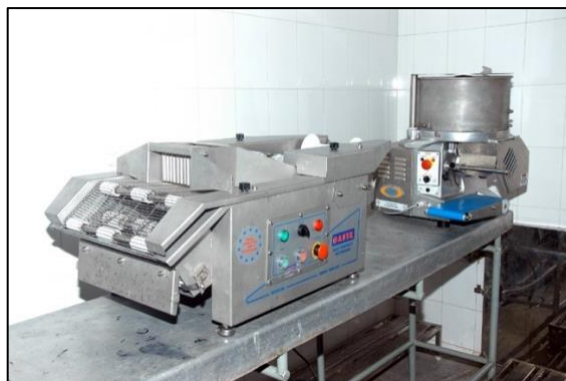
Battering and breading machine
