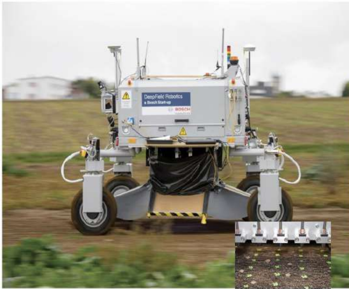
This robot is designed to work fields on its own and mechanically kill weeds. Photo: Deepfield
