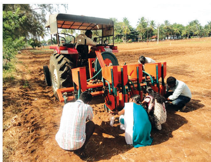
d) CIAE tractor-drawn pneumatic planter (T4)
