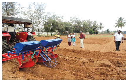
c) TNAU tractor-drawn ridger seeder (T3)
