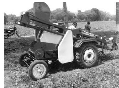
Fig. 1 Commercially available groundnut combine
