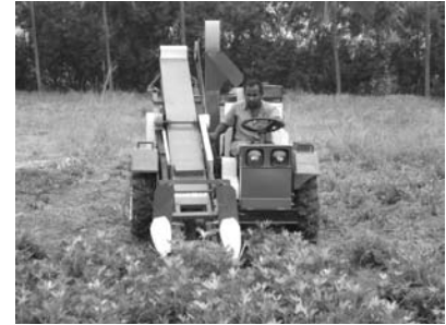
Fig. 4 Operational view of groundnut combine
