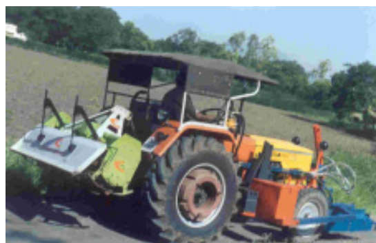
Fig.1. Tractor operated cotton stalk shredder cum insitu applicator
