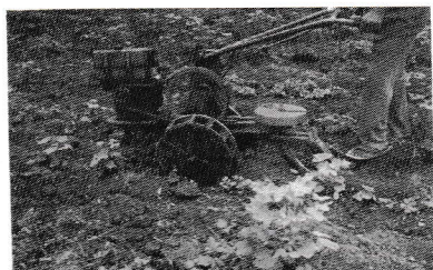
Fig.2 Self propelled power weeder.
