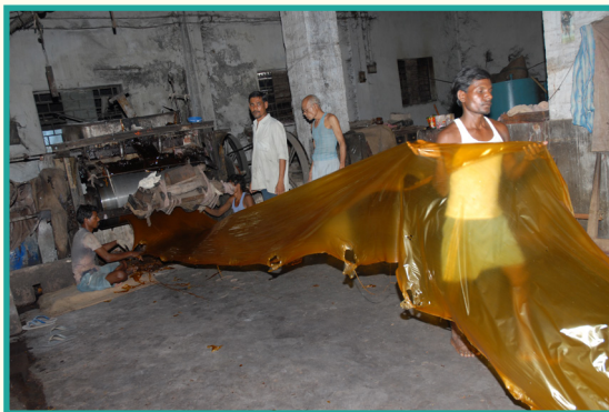
Photo 1. Preparation of the machine made shellac
