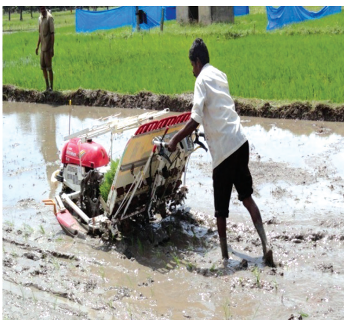
Fig. 3. Self propelled walk behind type transplanter
