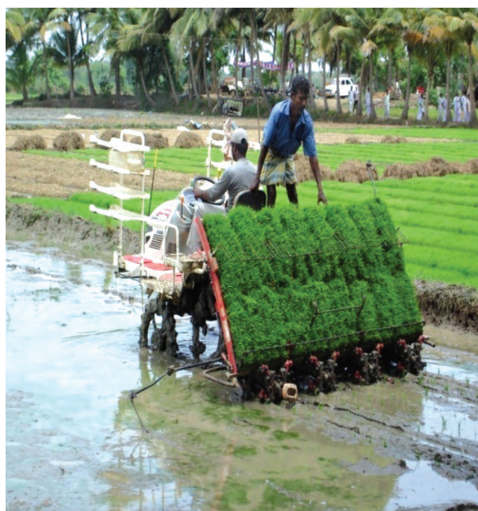
Fig. 4. Self propelled riding type transplanter
