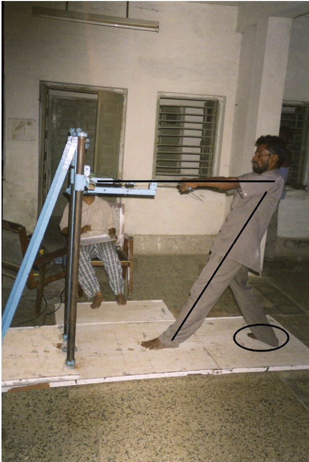
Fig. 2. Measurement of pull force with both hands in standing posture in horizontal plane.
