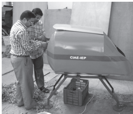
Fig. 5 Evaluation of power operated curry leaf stripper
