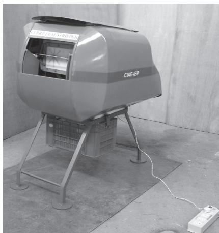
Fig. 4 Power operated curry leaf stripper
