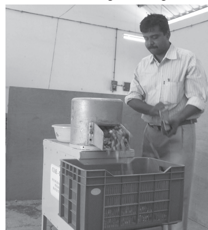
Fig. 10 Continuous long trials of batch type multiplier onion peeler with centrifugal discharge
