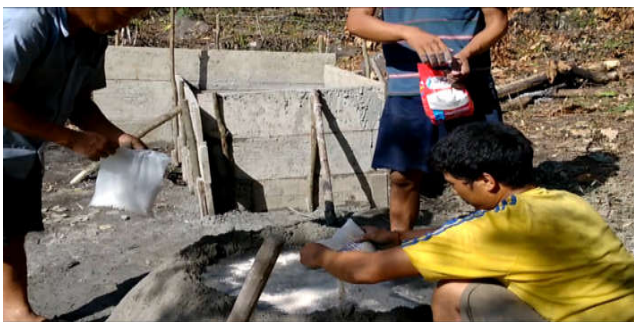
Fig 7 Preparing mixture of Salt, Mineral Mixture, Cement and Fine Sand in ratio (1:0.05:1:3)
