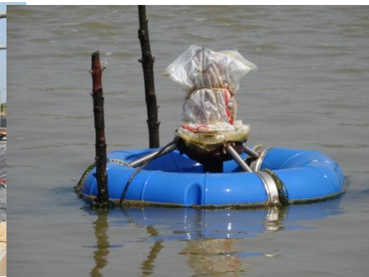
Round flow pond aerator
