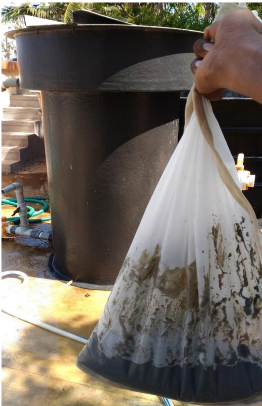
Fig 2. Harvesting of bioflocs using radial settler
