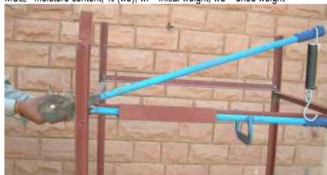
Fig-2 Setup for measuring cutting force and energy requirement for henna stem
