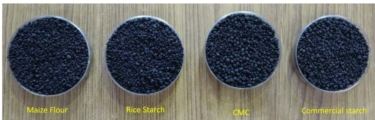
Fig. 3: Biochar pellets prepared using different binding materials
