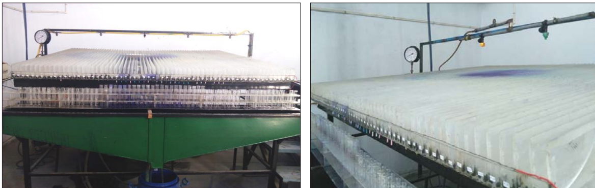
Fig. 3: Nozzles attached at the centre of the adjustable frame over the patternator
