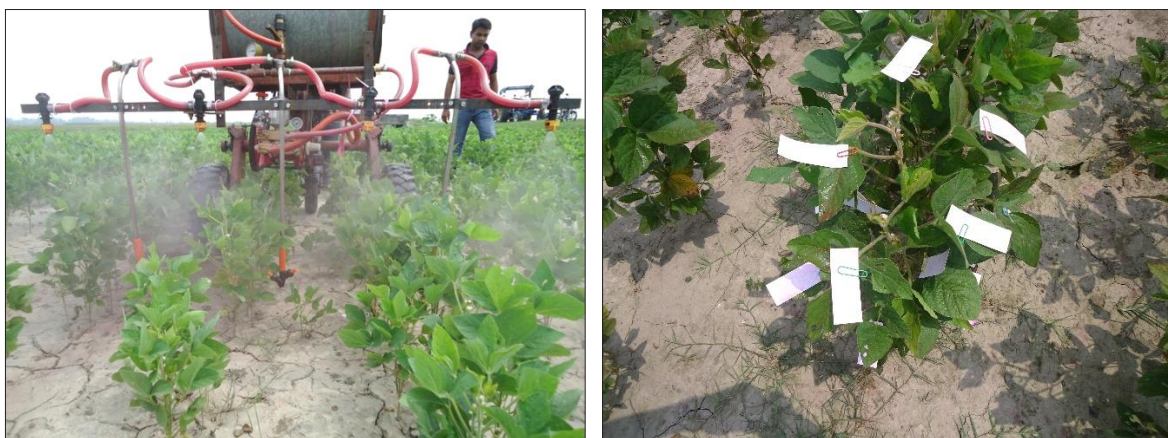
Fig. 4: Field performance evaluation of self-propelled boom spraying system in soybean crop
