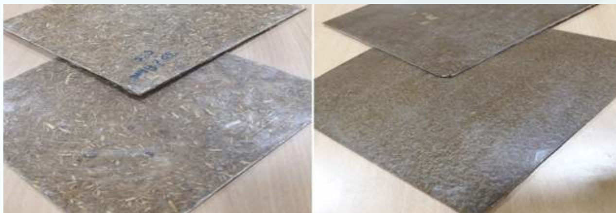
Fig. 2.14 Epoxy resin composites impregnated with cotton stalks and NLC prepared from cotton stalks
