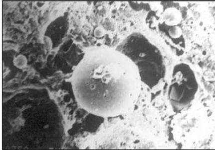
b. Control formulation showing the latticed structure (x 4000)
