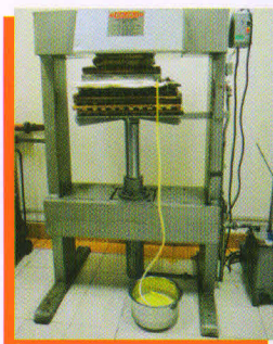
Juice extraction by Hydraulic Press
