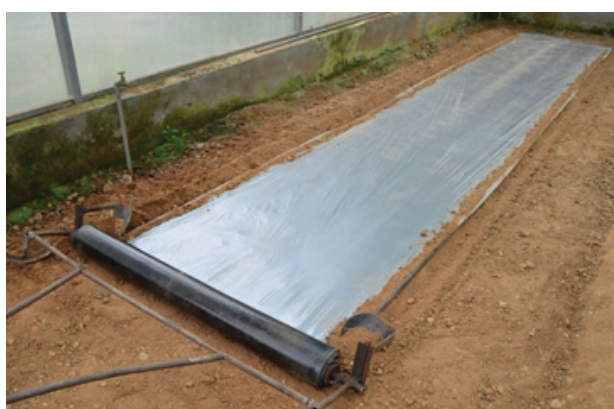
Manual mulch laying machine after satisfactory operation
