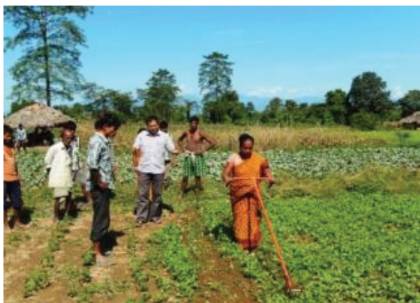
Fig.1. Twin Wheel Hoe under operation
