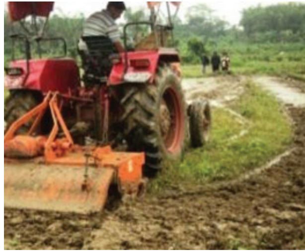
Fig: 2. Rotavator operation under wet land condition.
