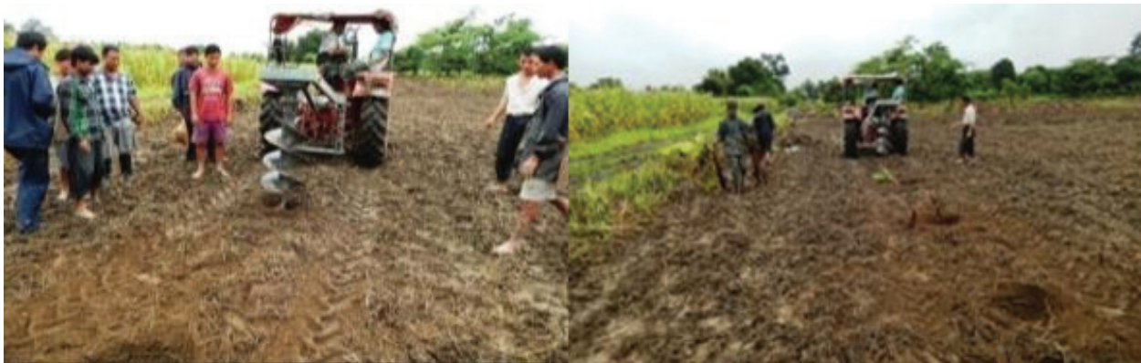
Fig.1. Operation of Tractor operated post hole digger for planting banana sapling.
