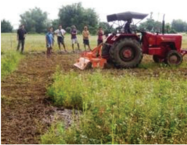
Fig: 1. Rotavator operation under dry land condition.
