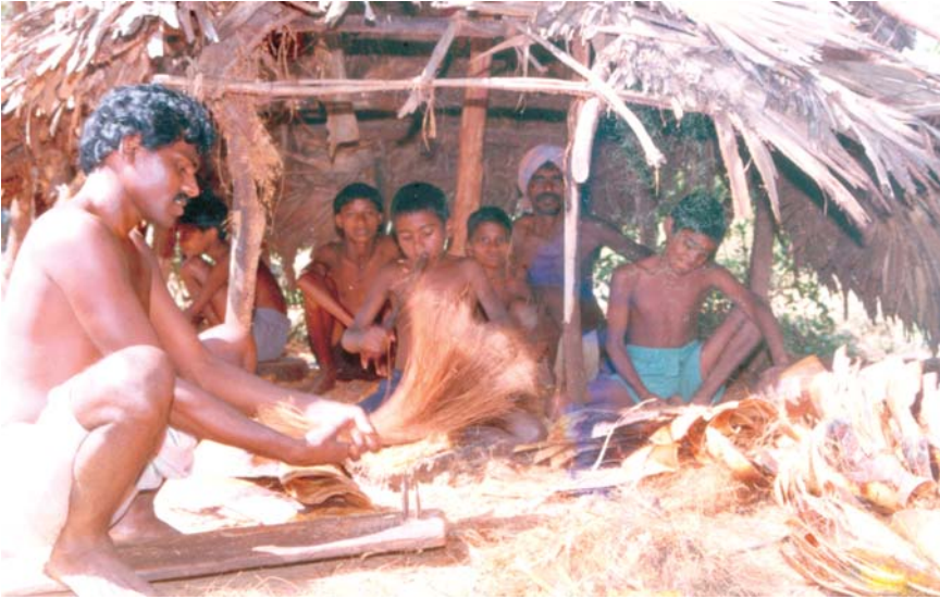
Manual extraction process - combing
