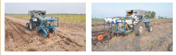
Fig. 5.3. Stubble shaving, Off-barring, Root pruning and Placement of basal dose of fertilisers
