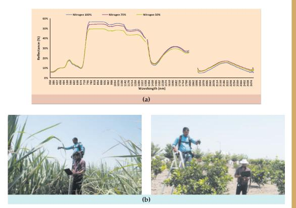
**Fig. 2.1.** Spectra of different levels of nitrogen in Sugarcane varitiey Co-10001 (a) and Hyperspectral data collection using ASD spectro-radiometer (b)
