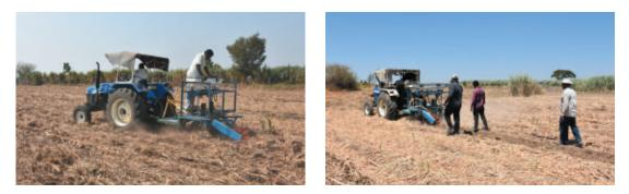
Fig. 2.34. Demonstration of stubble shaver, off-bar, root pruner cum fertilizer drill (SORF) machine at farmer's fields
